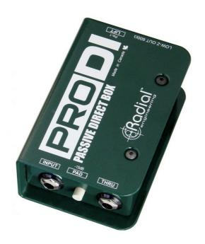
The ProDI is a passive direct box designed for use on stage or in home recording studios, with the ability to handle high output instruments without distortion, and a transformer-isolated output to eliminate noise from ground loops.<br/>
