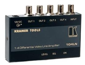
This is a unique piece of equipment that combines the functions of a distribution amplifier and a line driver. It accepts one composite video input and distributes a signal to four buffered outputs; gain and EQ controls are used to adjust the output level and equalization. The controls are used to compensate for signal losses in such situations as long cable runs. This model offers a differential input for noise elimination.
