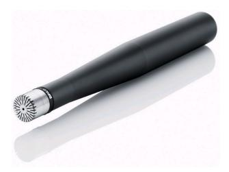
The mic is a phantom powered (P48) close miking specialist with an extremely linear on-axis response in an extended frequency range from 10 Hz to 40 kHz (±2 dB). This microphone is suitable for a wide range of applications from AB stereo pair to close-miking tasks as well as measurement requirements.
