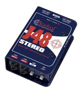
The J48 stereo is a high performance 2-channel active direct box for live concert touring and professional recording studio applications, with the ability to handle extreme transients without distortion while delivering the natural sound of your instrument.<br/>
