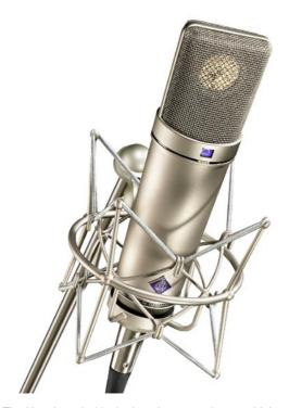
The U 87 is probably the best known and most widely used Neumann studio microphone. It is equipped with a large dual-diaphragm capsule with three directional patterns: omnidirectional, cardioid and figure-8. These are selectable with a switch below the headgrille. A 10 dB attenuation switch is located on the rear. It enables the microphone to handle sound pressure levels up to 127 dB without distortion. Furthermore, the low frequency response can be reduced to compensate for proximity effect.
