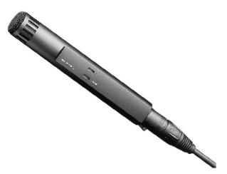
The super-cardioid MKH 50 offers a higher attenuation of diffusefield and lateral sound than the cardioid microphone. It is principally designed for use as a soloists or spot microphone for applications requiring a high degree of side-borne sound muting and feedback rejection. The directional characteristics are frequency-independent.
