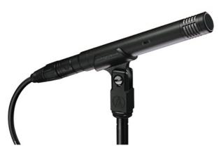
This premium electret condenser microphone is engineered to meet the most critical acoustic requirements of professional recording, broadcast and live sound. The AT4041 cardioid studio condenser microphone features a smooth, extended frequency response with a slight rise in the high-frequency region and a transformerless output for very high SPL-handling capability.
