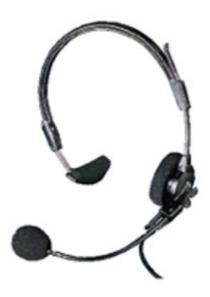
The PH-88 is a single-sided lightweight headset offering wearing comfort over extended periods. It has a dynamic noise-cancelling gooseneck microphone with a semi-rigid, fully adjustable boom for precise positioning. The high-quality wide band dynamic earphones are covered in moleskin for superior fit, isolation and frequency response. Earphones 300 ohms, microphone 200 ohms.
