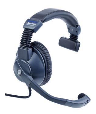
The CC-95 is a single-ear enclosed headset that offers the same full range audio response, acoustic isolation, comfort and durability as the CC-260. The 270 degrees boom rotation offers the user the option of left or right ear operation.
